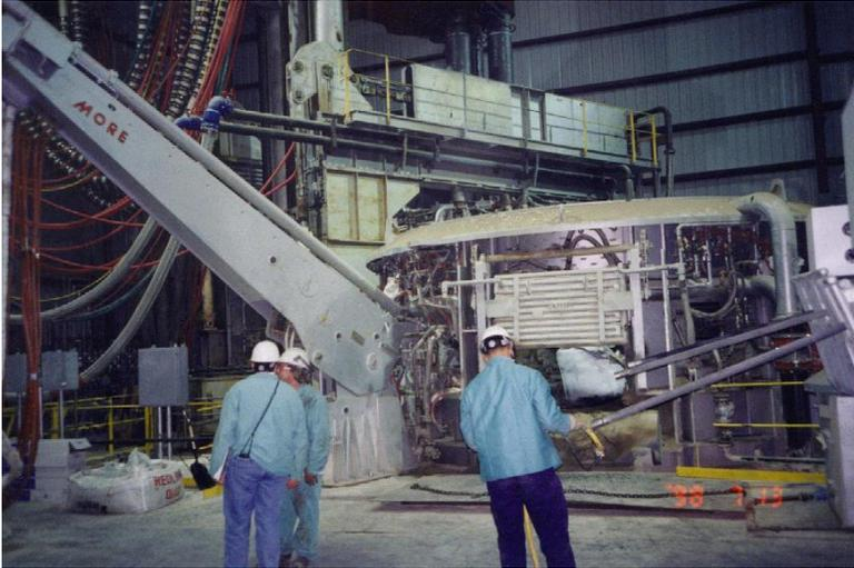
Figure 3 – Qualitech Steel Injecting Iron Carbide into an EAF at Pittsboro, Indiana, 1998
