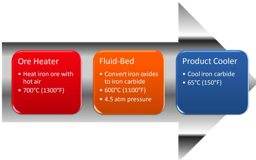
Figure 1 – Iron Carbide Simplified Manufacturing Process
