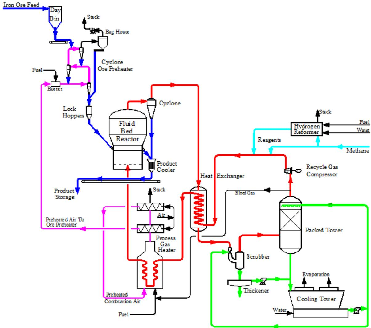
Figure 2 – Iron Carbide Process Flow Diagram
