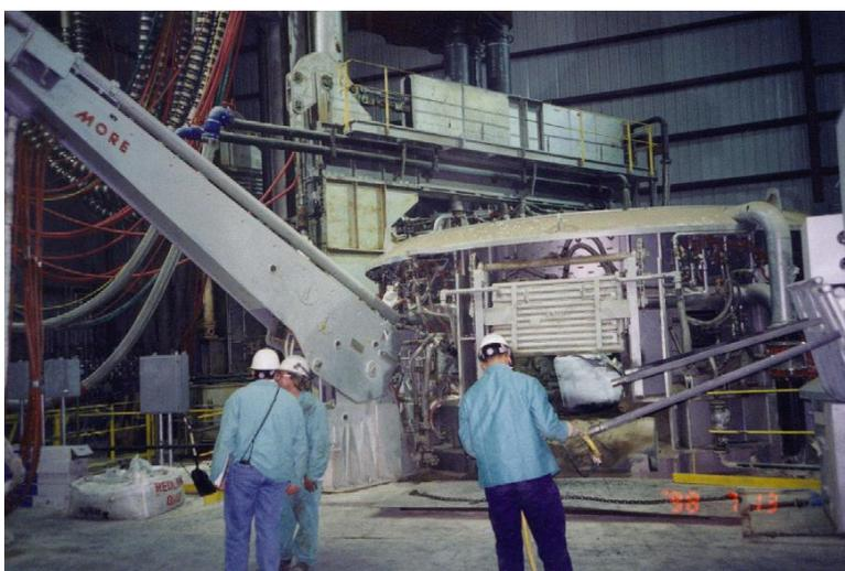
Figure 1. Qualitech Steel Injecting Iron Carbide into an EAF at Pittsboro, Indiana, 1998
