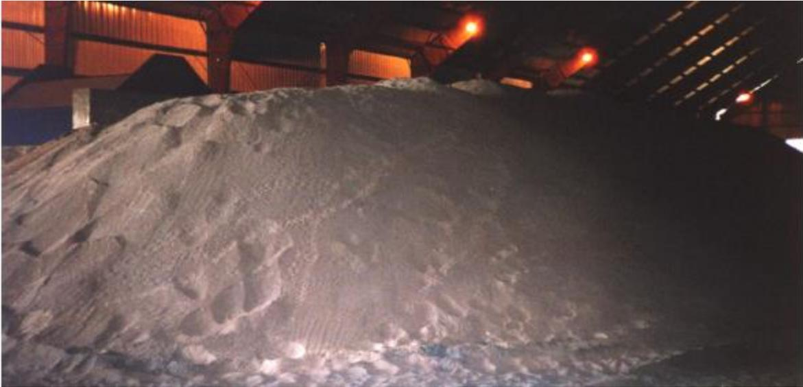
Fig.9: Part of the first iron carbide produced in the Nucor plant, Trinidad. (Photo Frank A. Stephens)
