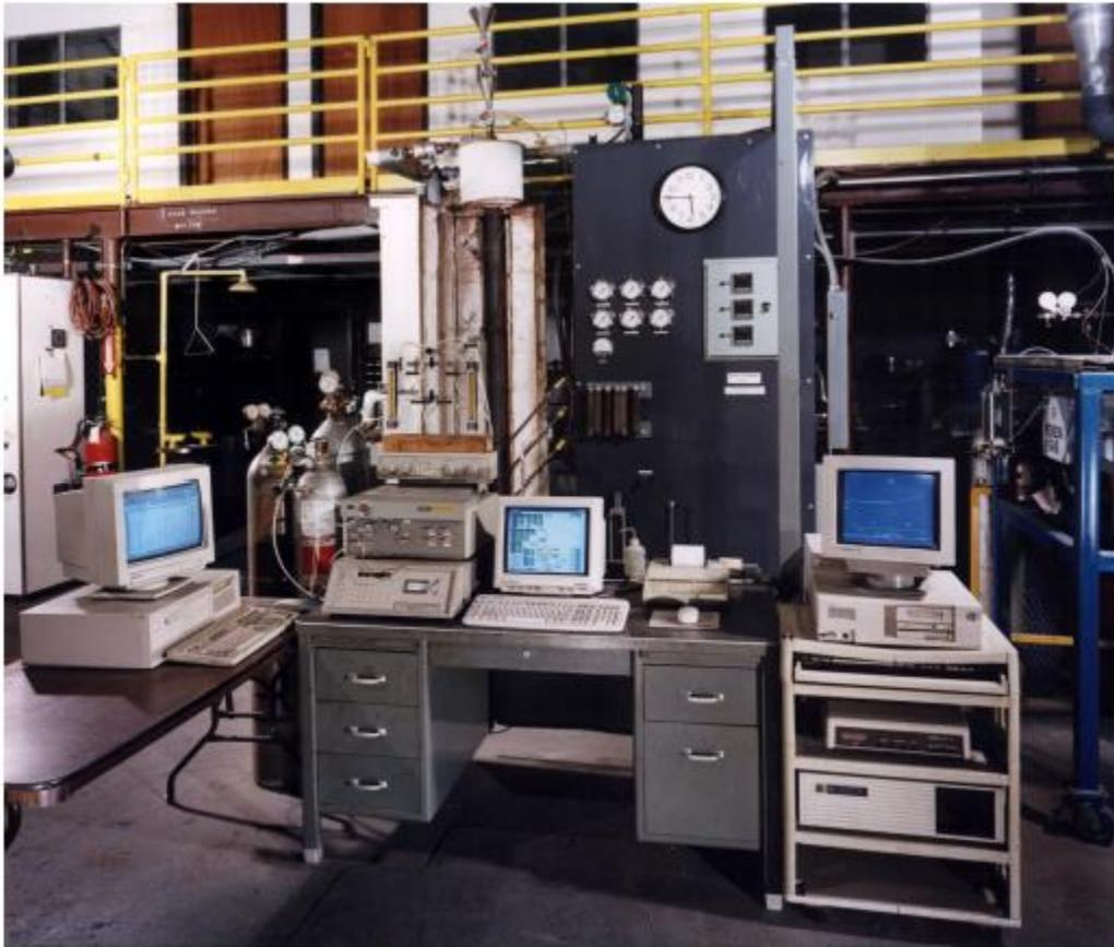
Fig.6: Equipment for the laboratory tests used at Hazen Research, Colorado, to assess and define the parameters for the production of iron carbide. (Photo Frank A. Stephens)
