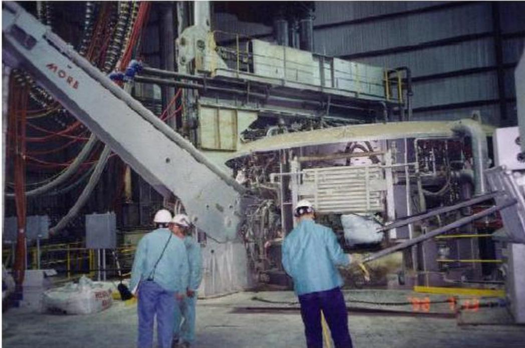
Fig.4: Qualitech Steel inject iron carbide in an EAF to Pittsboro, Indiana, 1998 [10]
